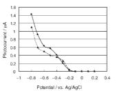
Langmuir-Blodgett films of purple membrane (PM) was prepared by application of DC electric field for orientation at the air-water interface and photocurrent was measured on gold electrode in aqueous KCl electrolyte. Dependences of steady photocurrent on electrode potential for PM films of DC-field applied preparation (solid line) and no field application (dashed line).
